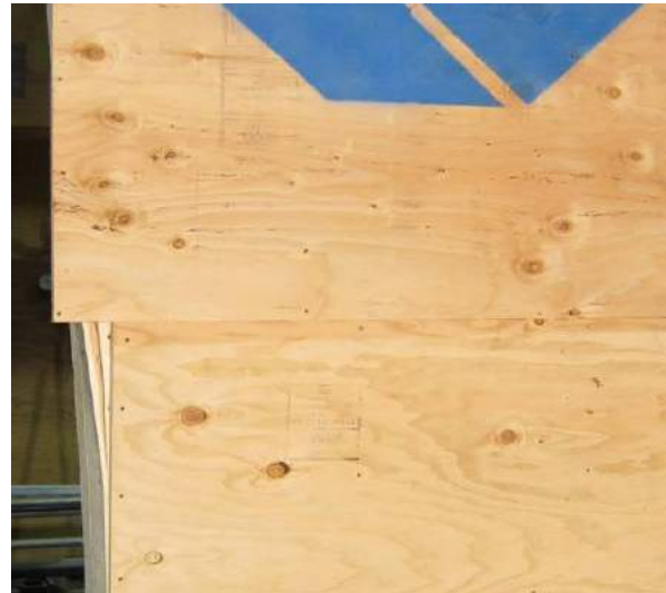
Figure 15 Pacific SmartWall® specimen failure
